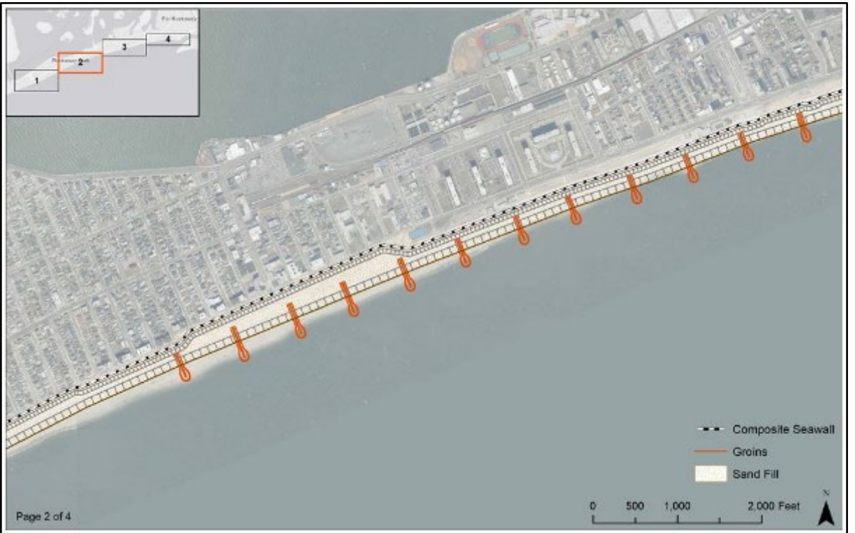
FIGURE 4.—Overview of ocean beach project features in the central part of the proposed project area. Illustration credit: USACE (2018a).
