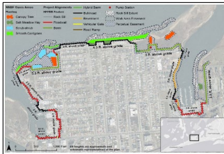
FIGURE 14.—Aerial photo with showing plan layout of Arverne Area HFFRRF. Illustration credit: USACE (2018a).
